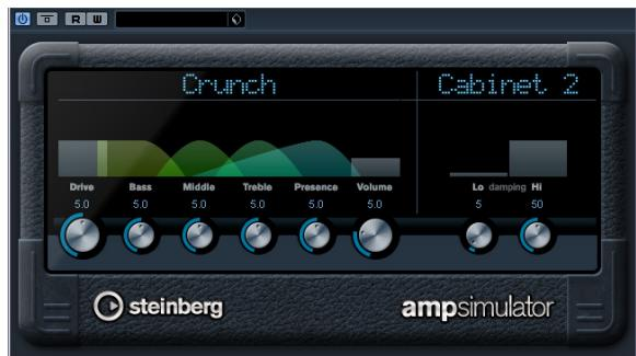
AmpSimulator is a distortion effect, emulating the sound of various types of guitar amp and speaker cabinet combinations. A wide selection of amp and cabinet models is available.
