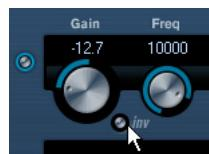
This is very useful if you want to filter out unwanted noise. While looking for the frequency to omit, it sometimes helps to boost it in the first place (set the filter to positive gain). After you have found this frequency, you can use the Inv button to cancel it out.
